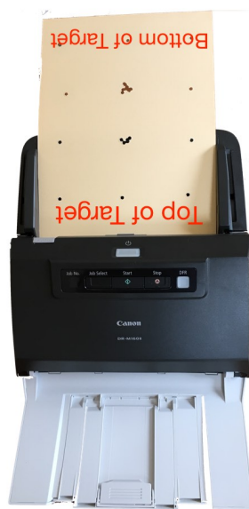
Figure 12: Targets are feed into the scanner upside down and the aiming bulls facing away.
